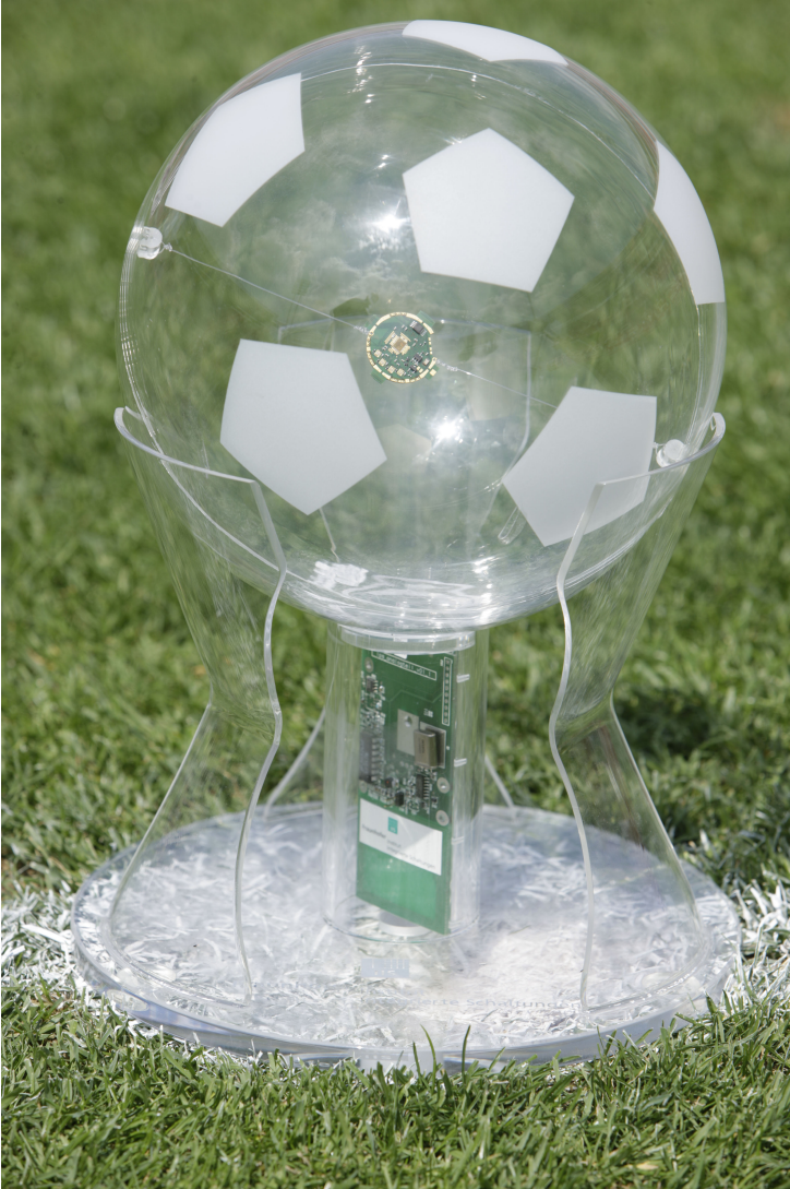
Figure 2.6.: A glass model of the ball's transmitter and inductive charger.
